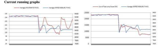
It is clearly visible from above and below curve that after a certain condensing load this phenomenon occurs. In this case when we tried to increase the condensing load above 66T/H the speed fluctuation appeared and LP control vale started oscillating .
